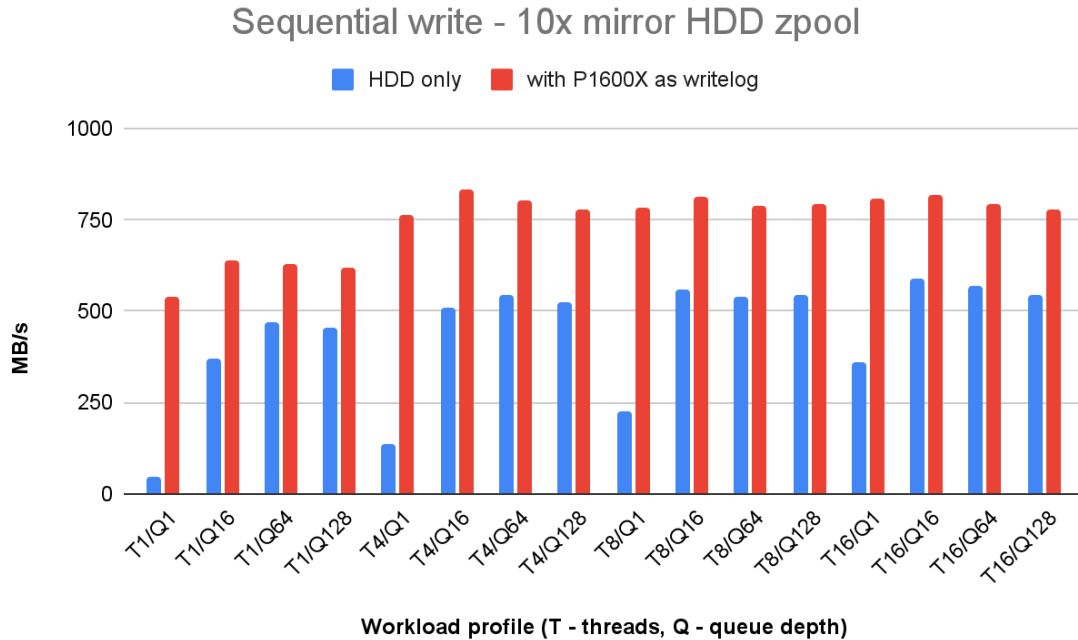
Fig. 13. Sequential write performance of a 10x mirror HDD zpool, with and w/o writelog.
