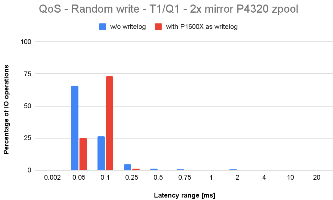
Fig. 23. Latency distribution for a random write test, done on a 2x 2-way mirror SSD zpool (T1/Q1), with and without writelog.
