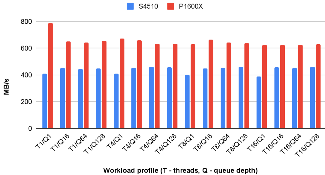
Fig. 8. Sequential write performance on a single boot medium, compared to the S4510.
