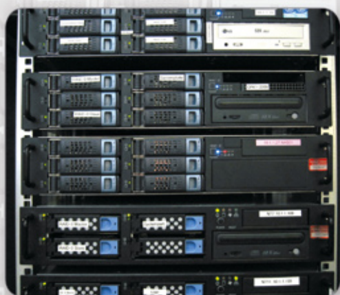
Using one Open-E NAS 2.0, the NAS01 storage array in the middle of the 19-inch rack makes all the patient records available to the hospital information system online via Gigabit Ethernet.
