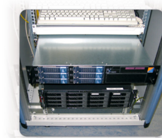
The Klinikum Oldenburg saves the data from the NAS01 storage array online onto the second storage array, which also controls an Open-E NAS 2.0, using Gigabit Ethernet.
