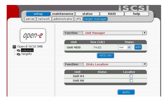
Next, the page will be reloaded, and status field will show your units as "in use" and with new group e.g. "vg0". The Volume Group is the equivalent of a physical disk from the system point of view. It is also possible to combine two (or more) units into one Volume Group by choosing one of actually existing groups like "vg0", or by choosing "new" option, which will create new group "vg1" after using "add" button.
