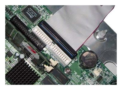
Every motherboard has at least two such ports. To install Open-E iSCSI, you have to use the first (primary) port.
