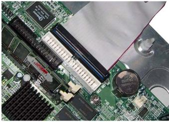
Every mainboard has at least two such ports. To install Open-E NAS SOHO, you have to use the first port because your computer "expects" this to be the position from which the booting process starts. In this example, this will soon be Open-E NAS SOHO.
